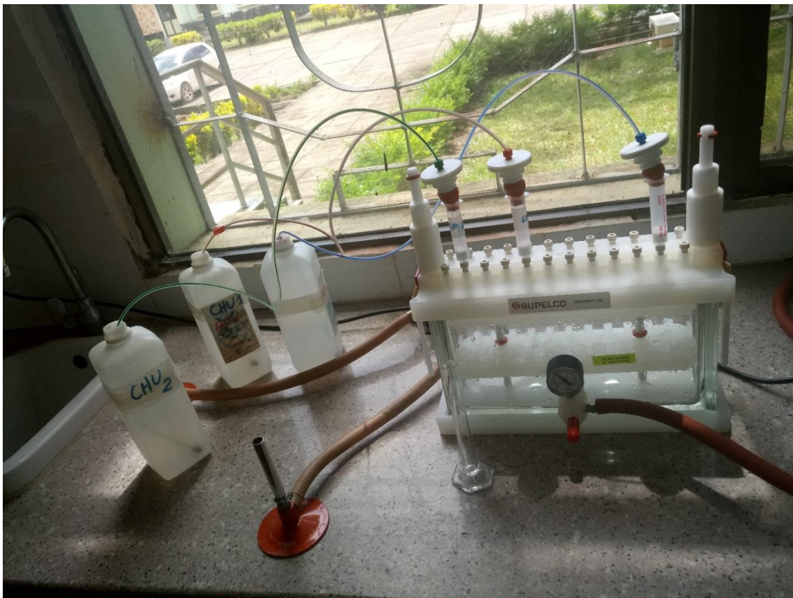
Figure 3.13: Solid Phase Extraction (SPE) as way of sample preparation before analysis
